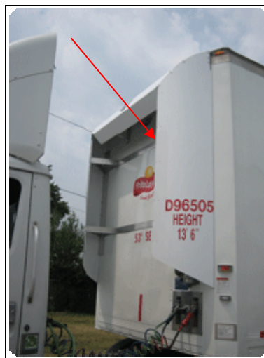
Figure 24: Example of gap fairing mounted to van semi-trailer
