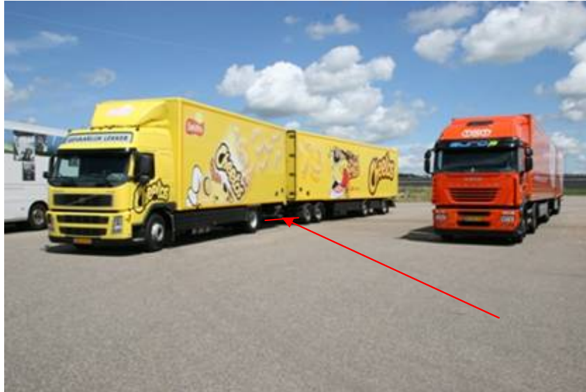
Figure 33: Example of gap in combination vehicles
