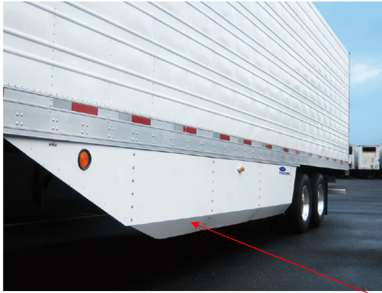
Figure 23: Example of belly fairing
