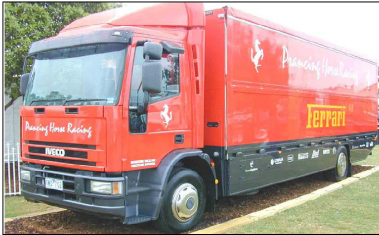
Figure 8: Example of bodywork that fulfills the sideguard regulation requirements [3]
