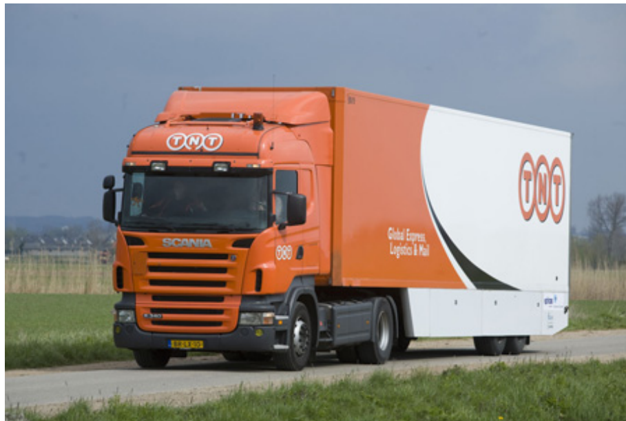
Figure 28: Example of rigid, continuous, flush fairing/side guard
