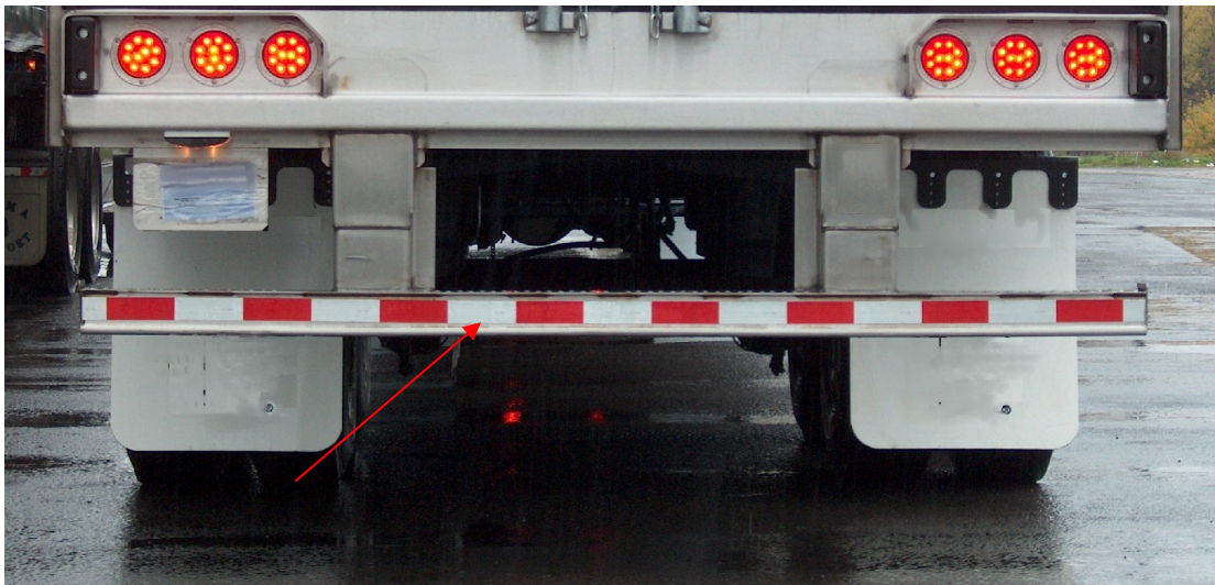
Figure 26: Example of rear underride guard
