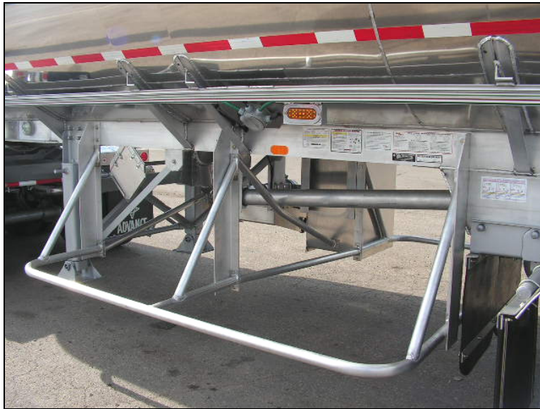
Figure 10: Close-up of a sideguard installed on a Canadian operated tanker trailer
