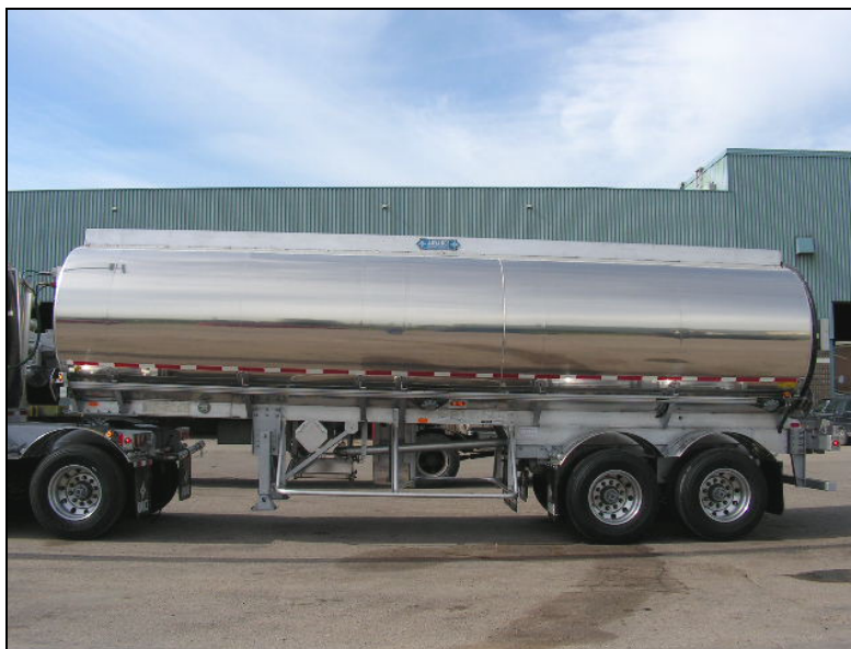
Figure 9: Sideguards installed on a Canadian operated tanker trailer
